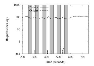
Figure 6: The WheelFS-based Web cache running on Emulab with failures, using the **.EventualConsistency** cue. Gray regions indicate the duration of a failure.
