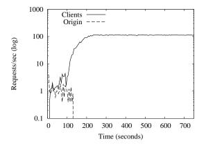
Figure 8: The aggregate client service rate and origin server load for the WheelFS-based Web cache, running on Emulab, without failures.
