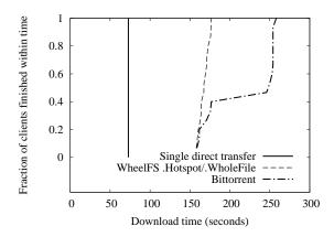
Figure 11: CDF of client download times of a 50 MB file using BitTorrent and WheelFS with the **.Hotspot** and **.WholeFile** cues, running on Emulab. Also shown is the time for a single client to download 50 MB directly using ttcp.
