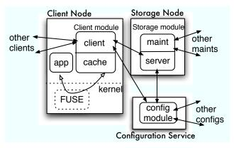
Figure 1: Placement and interaction of WheelFS components.
