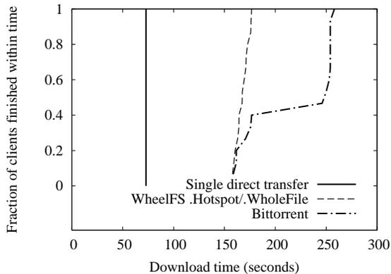
Figure 11: CDF of client download times of a 50 MB file using BitTorrent and WheelFS with the **.Hotspot** and **.WholeFile** cues, running on Emulab. Also shown is the time for a single client to download 50 MB directly using `tcp`.
