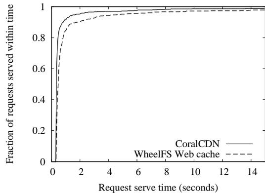
Figure 5: The CDF for the client request latencies of both CoralCDN and the WheelIFS-based Web cache, running on PlanetLab.
