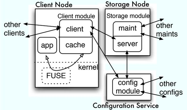
Figure 1: Placement and interaction of WheelFS components.
