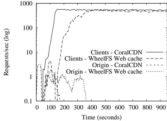
Figure 4: The aggregate client service rate and origin server load for both CoralCDN and the WheelIFS-based Web cache, running on PlanetLab.
